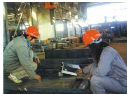
Ultrasonic test 探伤
